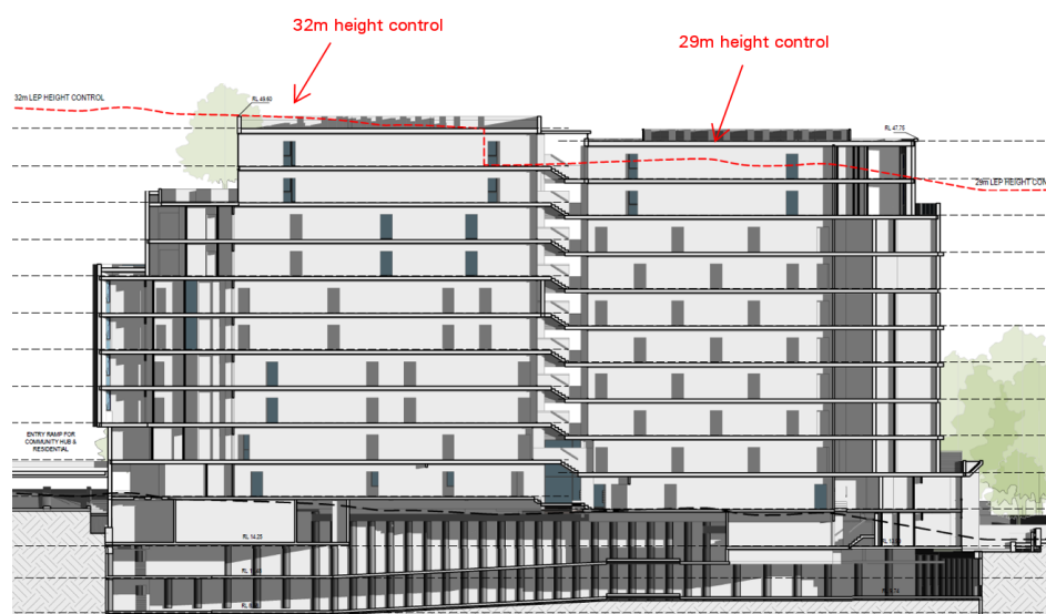
Figure 6 – Building A1 and A2 Maximum Height Source: Mirvac Design
